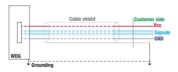
L2/L3, T3: Cable shield connected to encoder housing. Encoder housing not earthed separately.
